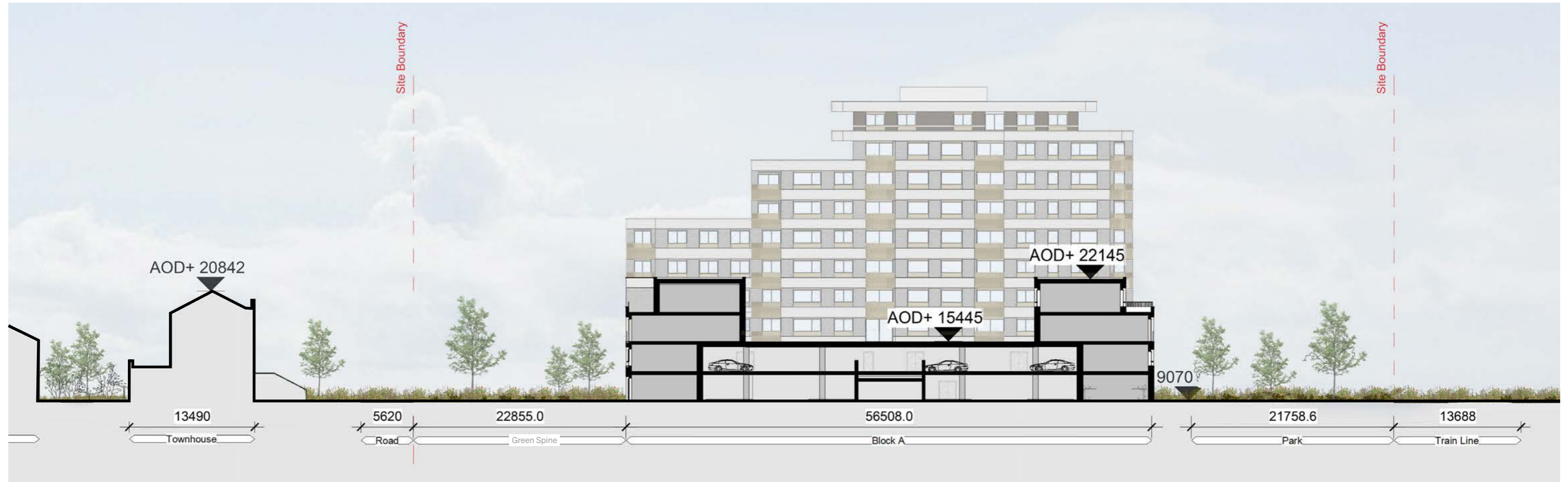
Fig. 34 Section from Phase 1 to the Trainline
