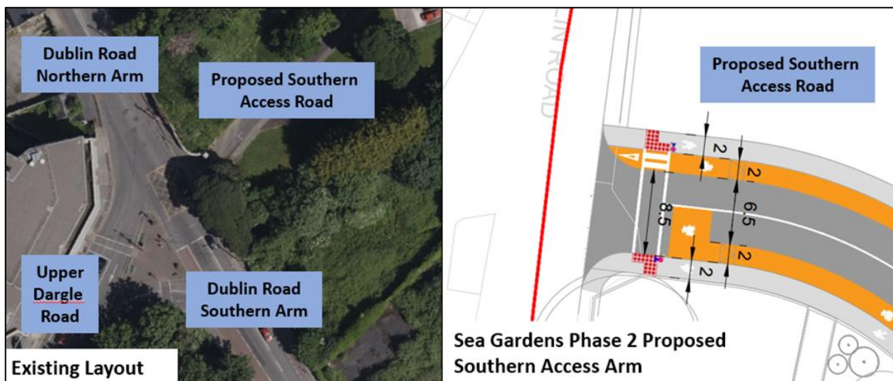
Figure 7-5 – Southern Access Road Junction Layout
