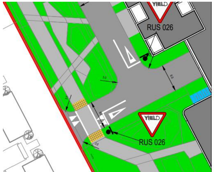
Figure 6-3 - Extract showing pedestrian priority at junction
