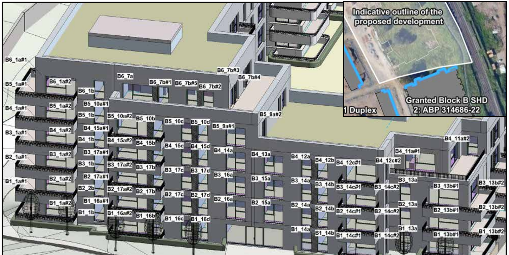
Figure A.5: Highlighted areas indicate the position of assessed windows (L), Aerial view of assessed location (R)
