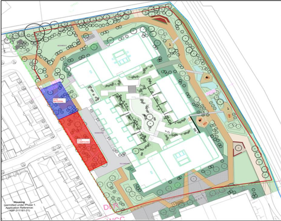
Figure 3-3 - Site Compound Location
